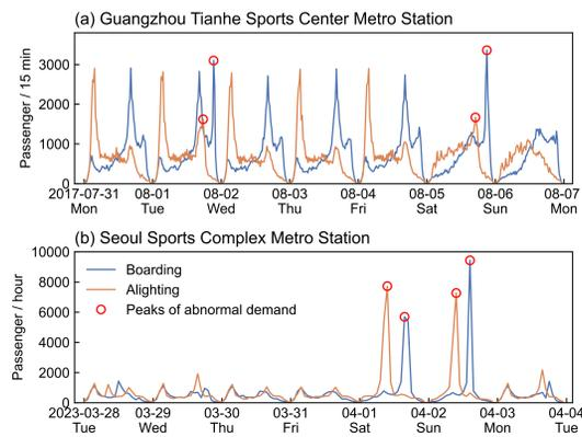
Figure 1. Passenger flow of two metro stations. Remarkably, a noticeable peak in abnormal alighting flow consistently precedes each peak in abnormal boarding flow.
