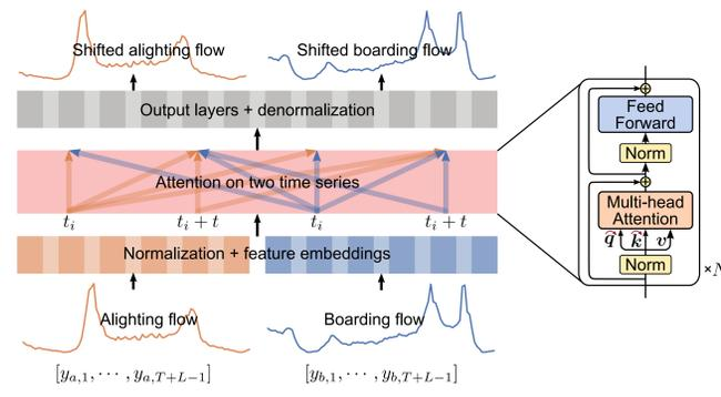
Figure 3. ABTransformer for metro passenger demand forecasting by explicitly modeling the correlations in the alighting and boarding flow.
