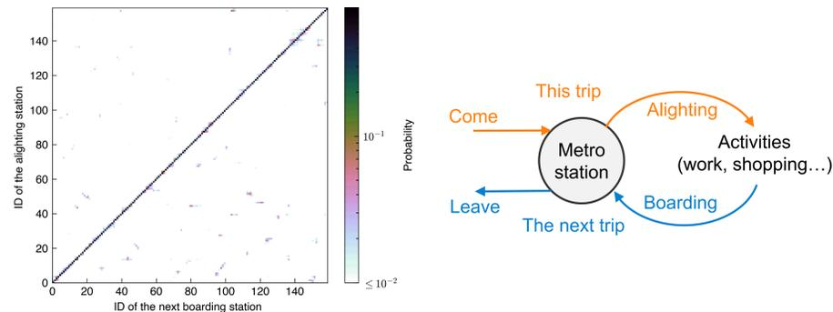
Figure 2. Illustration of alighting and boarding (AB) correlation. Left: The probability of the next boarding station given the current alighting station (Guangzhou metro data). Right: An illustration of chained behavior in metro systems.
