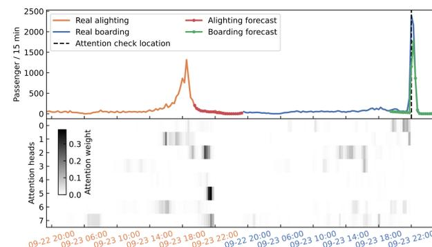
Figure 4. Interpreting boarding demand forecasting in a metro station in Guangzhou using attention weights of the last layer in the ABTransformer. The boarding demand forecast at the checked location exhibits significant attention to periods with abnormal alighting demand, indicating the parts of the input sequence that contribute to the forecast at the checked location.
